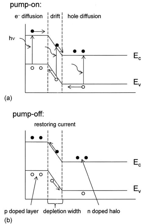
FIG. 1. Schematic energy band diagram of a  $p$ -type USJ for (a) pump laser on and (b) pump laser off. Carrier recombination and tunneling effects are not included here for clarity.
