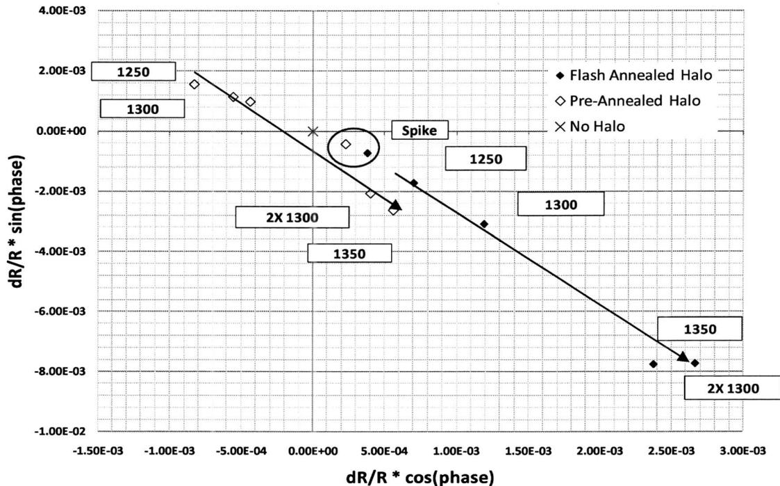
Fig. 2. Measured photorefectance vector for the USJ halo-doped samples (no PAI).
