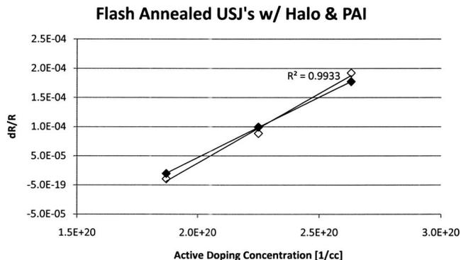
FIG. 6. PR signal plotted vs activation levels for the USJ halo-doped samples with PAI.
