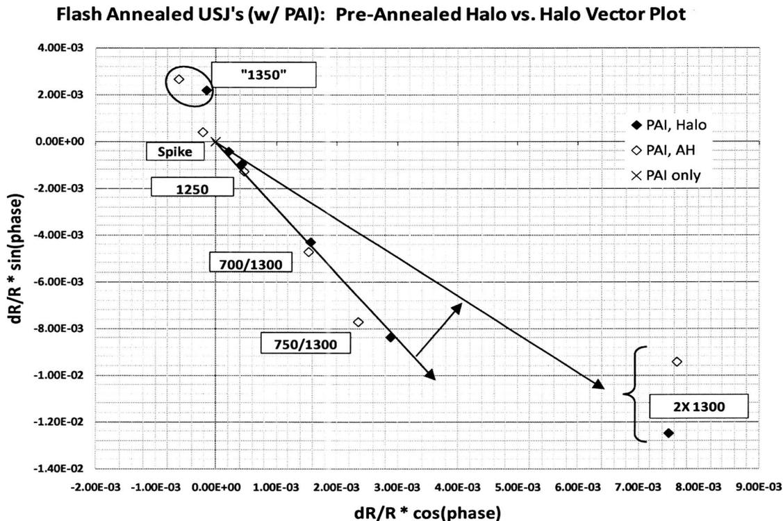
FIG. 4. Measured photorefectance vector for the USJ halo-doped samples with PAI.
