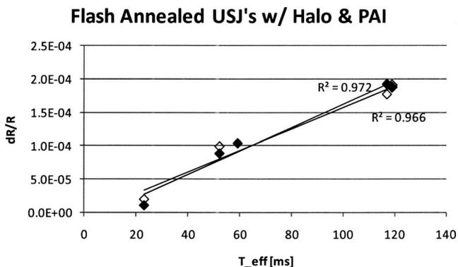
FIG. 5. PR signal plotted vs flash effective annealing time.
