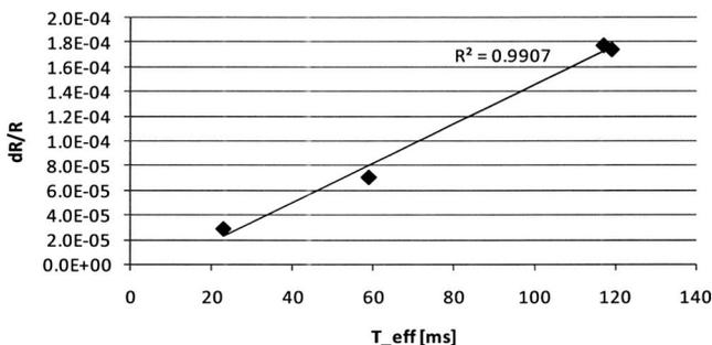
Fig. 3. Photorefectance signal plotted vs flash effective annealing time.
