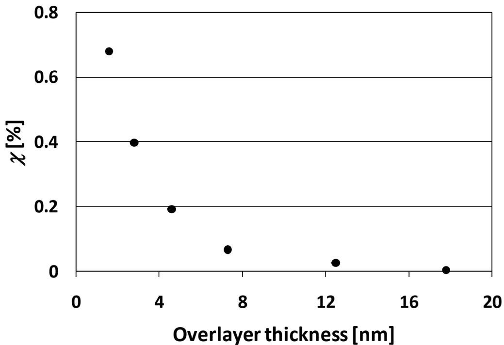
**FIGURE 4.** Strain in silicon overlayers derived from laser PR measurements.
