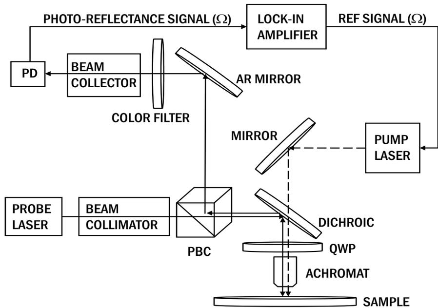
FIGURE 1. Schematic of laser PR apparatus.
