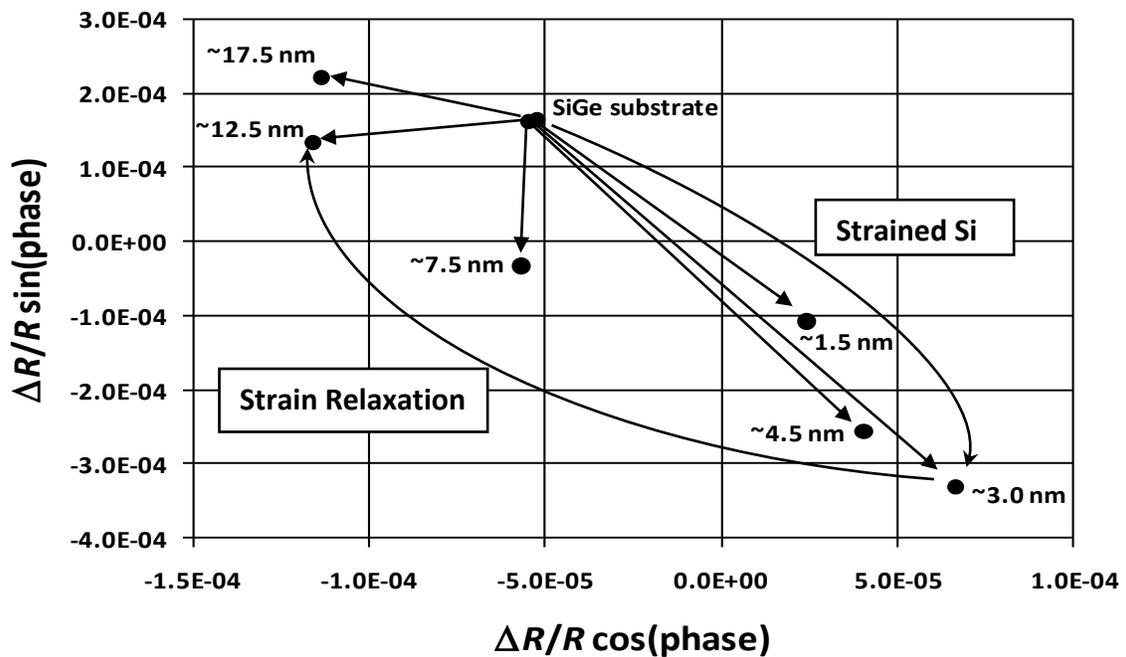
FIGURE 2. Laser PR signal from strained silicon on silicon-germanium substrates (after Ref. 10).
