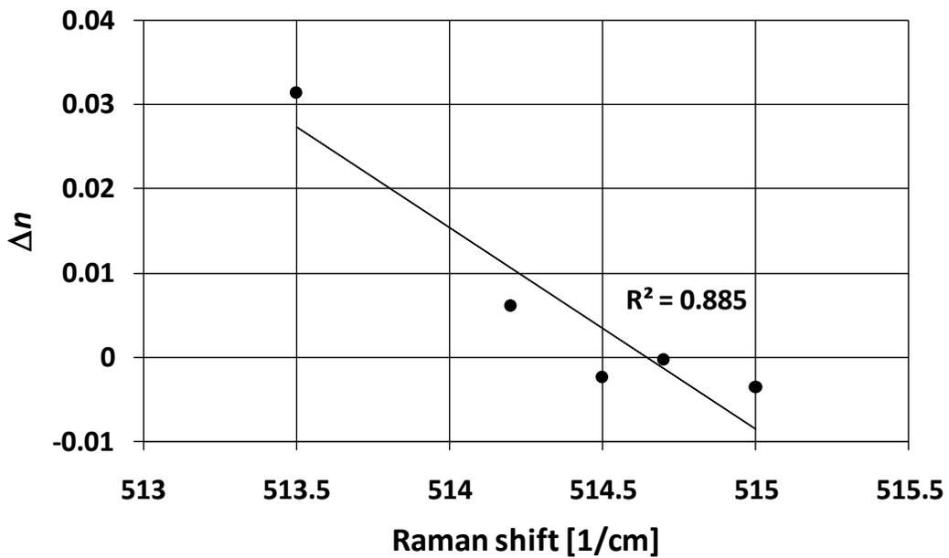
**FIGURE 3.** Comparison of nonlinear refraction with Raman shift of the LO phonon in Si.
